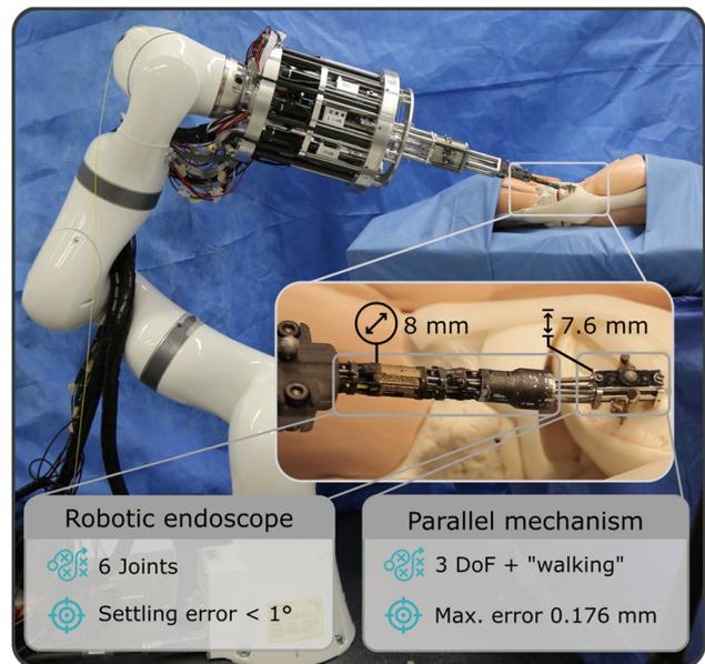
**Figure 3:** Overall mechanical system setup prototype.
