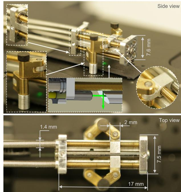
**Figure 2:** Miniature parallel mechanism for minimally invasive laser guidance.
