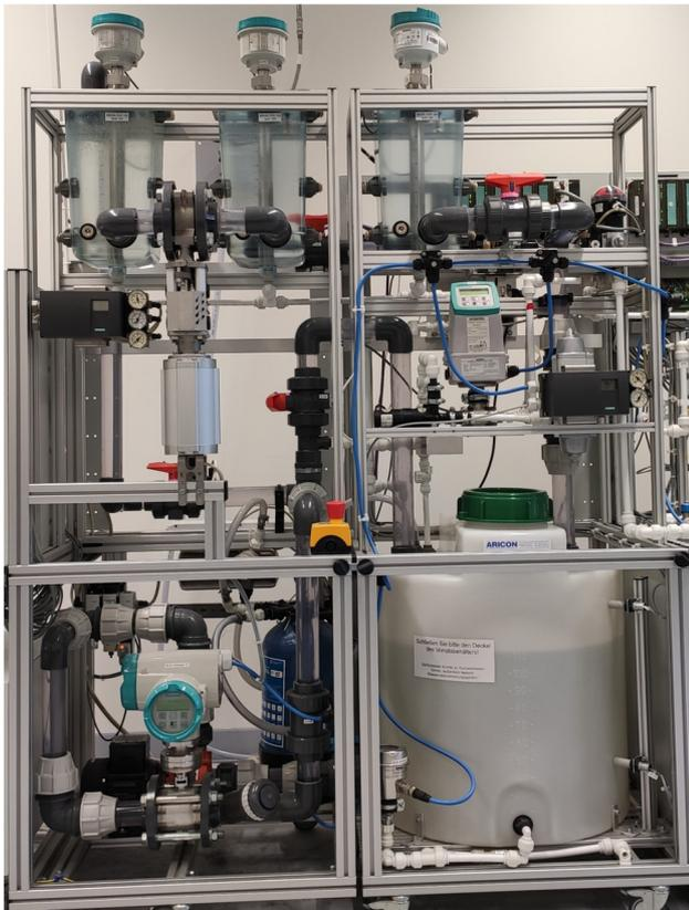
**Figure 6:** Experimental setup: The top three tanks correspond to tanks B2, B3, and B4 (from left to right). The black boxes in the middle of the image are the pneumatic valves  $V_1$  and  $V_6$  (from left to right). At the bottom of the picture are the pump and the reservoir tank B1.
