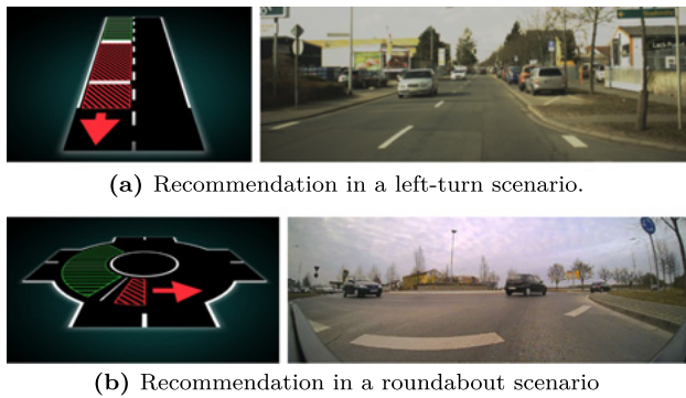
Figure 8: Recommendations for maneuver execution in the main HMI of the City Assistant System (left) with an image of the respective situation (right): The red arrow recommends to let the oncoming/crossing traffic pass. The dynamic visualization of gaps helps the driver anticipate the arrival of the “green” and thus sufficiently large gap.
