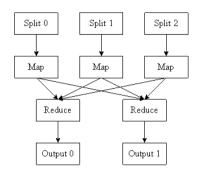
Figure 3: MapReduce calculation model
