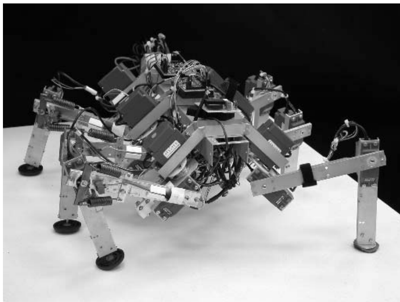
Figure 1 Robot TARRY: Walking based on biology-inspired algorithms.
