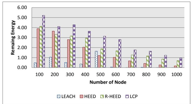
Fig.5. Total remaining energy in LCP in comparison with HEED, R-HEED.
