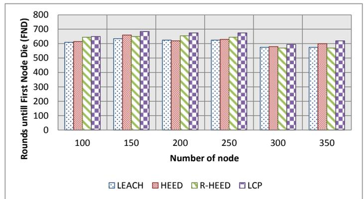
Fig.6. Comparing LEACH, HEED, R-HEED and LCP using different number of nodes for FND metric.
