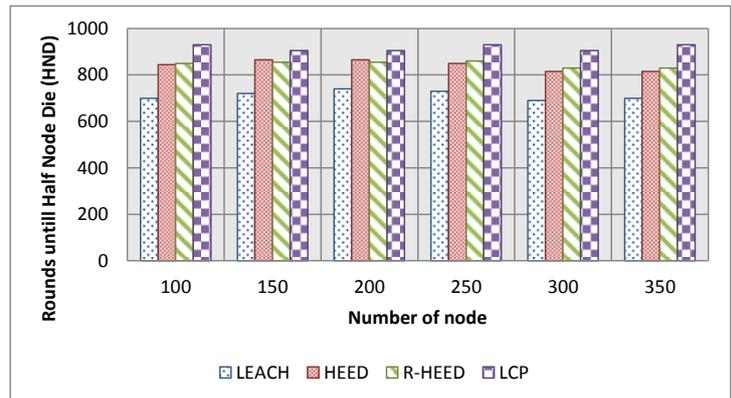
Fig.7. Comparing LEACH, HEED, R-HEED and LCP using different number of nodes for HND metric.
