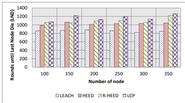
Fig.8. Comparing HEED and R-HEED using different number of nodes for LND metric.
