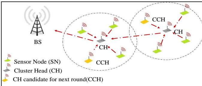
Fig.3. A Load-balancing Cluster Based Protocol Rotate phase.
