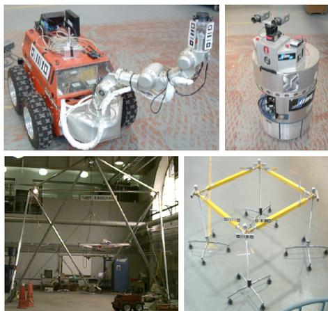
Fig. 1. The Mobile Manipulator (top left), the Roving Eye (top right), the Crane (bottom left) and the completed structure (bottom right).
