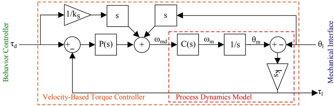
Fig. 4: Velocity-based SEA control system model.
