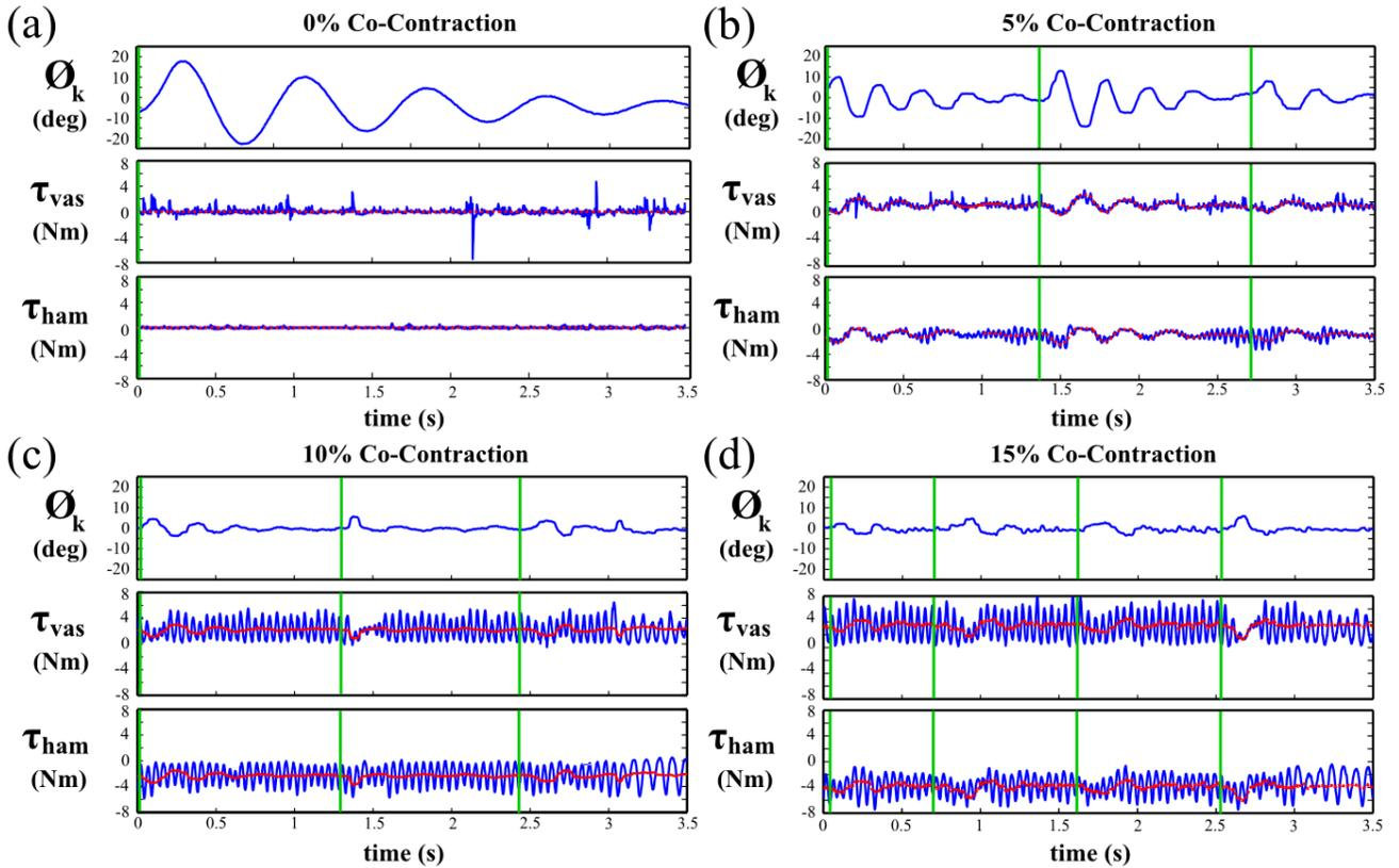
Fig. 6: RNL knee position and antagonistic actuator torque during co-contraction experiments for (a) 0% (b) 5% (c) 10% (d) 15%. Red lines: commanded trajectory. Blue lines: measured trajectory. Green lines: External impulse disturbances to instigate shank oscillation.
