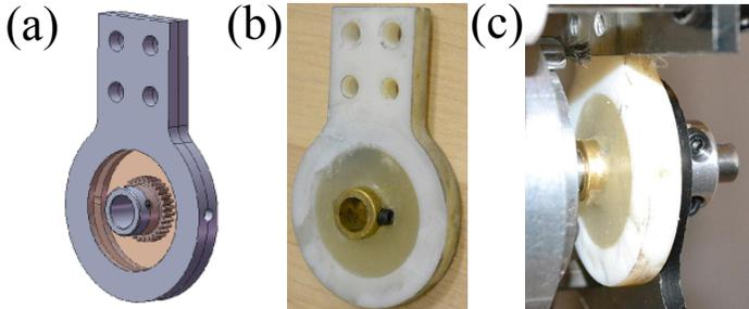
Fig. 3: Floating compliant knee joint. (a) Concept (b) Prototype (c) Close-up of implementation
