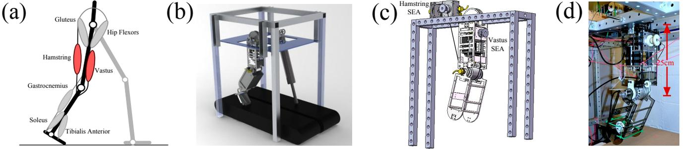
Fig. 1: Robotic testbed development. (a) Major human leg muscles with monoarticular knee extensor and biarticular knee flexor highlighted. (b) Testbed concept. (c) CAD assembly of initial stage. (d) Robotic implementation. For experiments, thigh was rigidly coupled to mounting cage.
