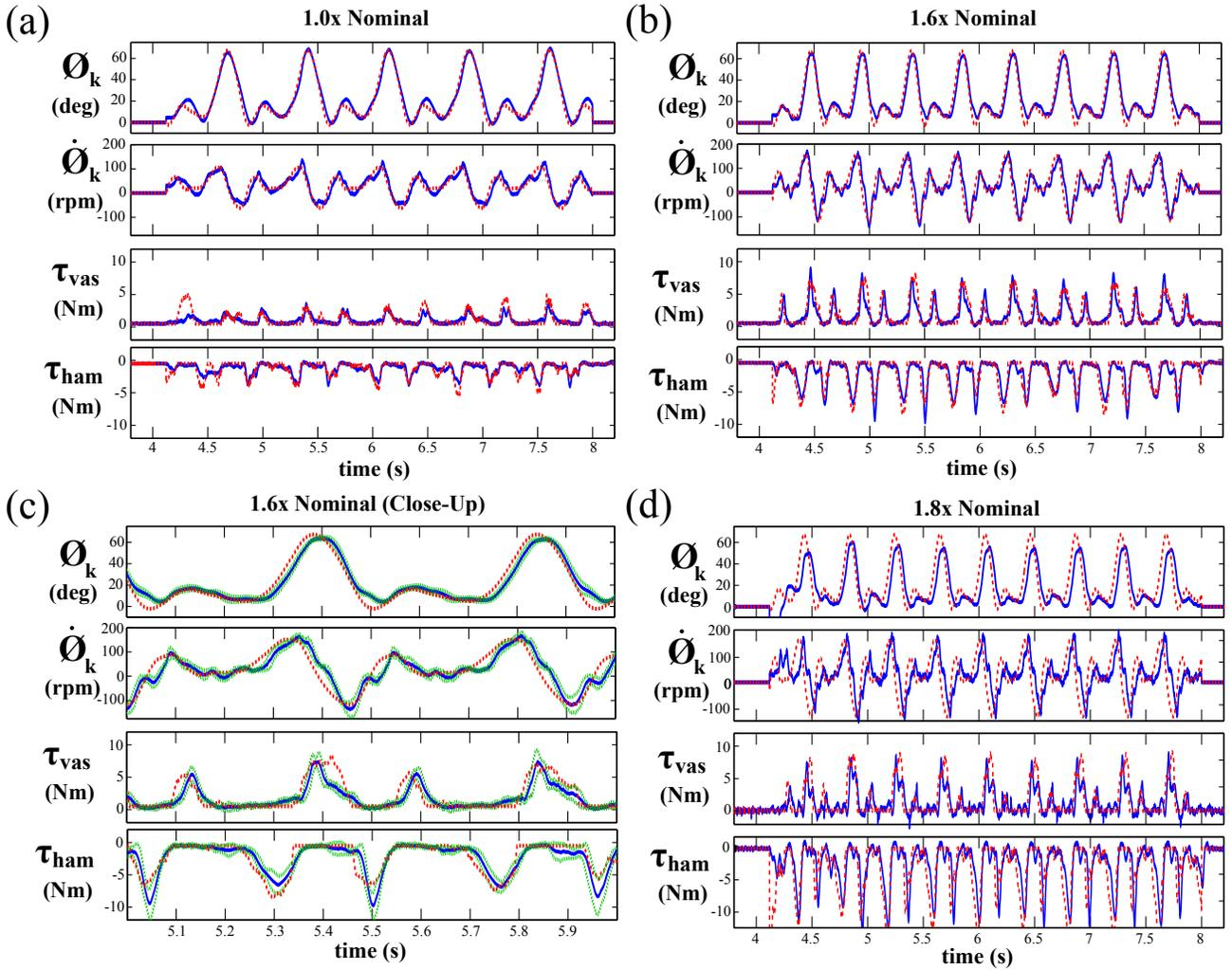
Fig. 5: High fidelity motion experiments. RNL knee position, velocity, and antagonistic actuator torques for walking trajectories corresponding to (a) 1.0x, (b,c) 1.6x, and (d) 1.8x nominal walking speed trajectories. In experiments, motion occurred between 4s and 8s. Plots show mean $\pm$ s.d. for 10 repetitions. Red lines: commanded trajectories. Blue lines: measured trajectories. Green lines:  $\pm$ s.d. of measured trajectories.
