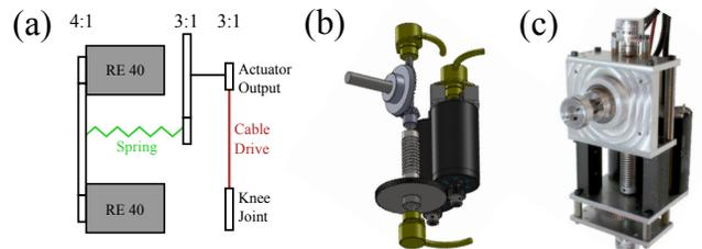
Fig. 2: RNL SEAs. (a) Drivetrain schematic (b) Drivetrain assembly (c) Prototype
