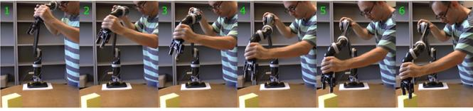
Fig. 3: Kinesthetic demonstration of reaching to an object (yellow box). Task-space pose of end-effector is used as input.
