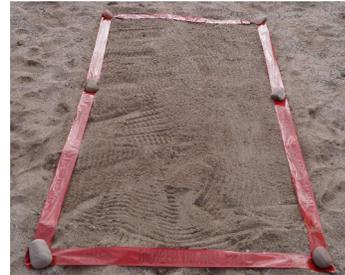
Fig. 9: The testbed in the Arizona desert used for evaluating and learning policies in a real environment. The surface of the testbed is flattened in order to increase comparability between the values measured for each policy.
