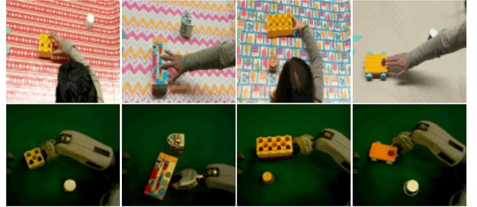
Fig. 8. Human and robot demonstrations used for meta-training for the experiments in Section VI-B with large domain shift. We used ten different diverse backgrounds for collecting human demonstrations.
