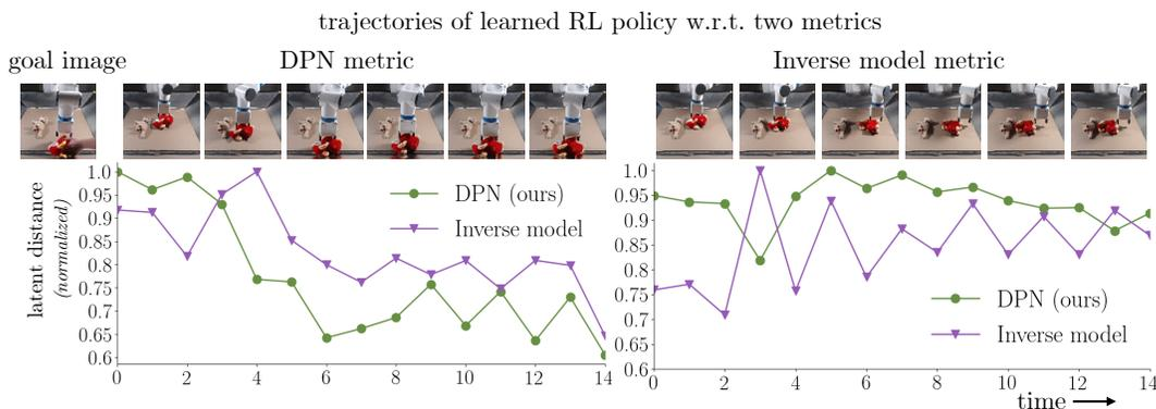
Fig. 6. Comparisons of normalized latent distance to the goal determined by DPN and inverse model for the real-world pushing task. We evaluate each latent metric on the trajectories of RL policy with respect to DPN and inverse model respectively, shown in the images above from left to right.
