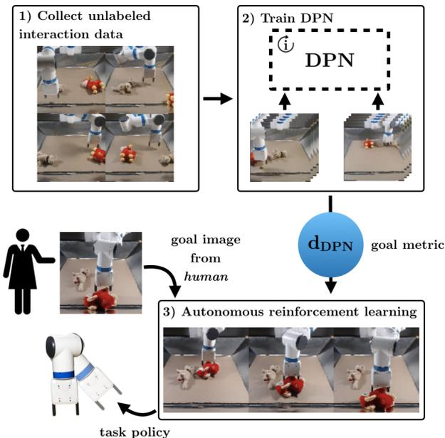
Fig. 1. General overview of our method. Our method, DPN, enables autonomous reinforcement learning, without human-provided reward functions, on vision-based manipulation problems.
