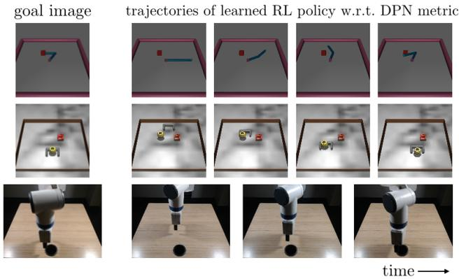
Fig. 7. Roll-outs of learned RL policy using the DPN metric of simulated reaching, simulated pushing, and robot reaching experiments from top to bottom.
