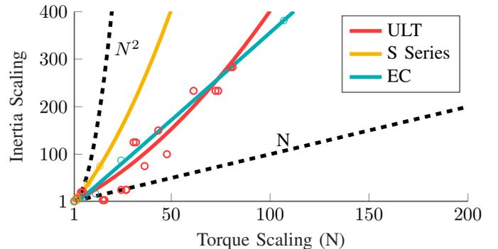
Fig. 3: Scaling laws for three commercially available motor series are compared against the  $N^2$  scaling law for gearboxes. The ULT series motors are manufactured by Celera Motion, the S series by Aerotech and the EC motors by Maxon.
