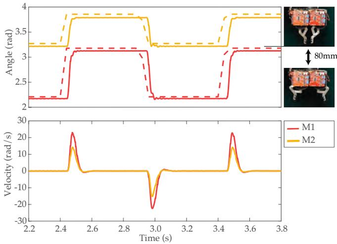
Fig. 6: A step response of one finger module of the DDHand showing the angular position and velocity of the motors. The dotted lines show the commanded positions. The delay seen between the command and response of the motor captures the round trip latency for CAN communication. The lack of an integral gain results in a small steady-state error.
