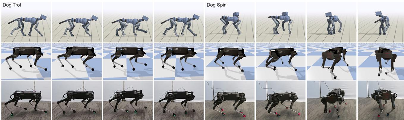
Fig. 1. Laikago robot performing locomotion skills learned by imitating motion data recorded from a real dog. **Top:** Motion capture data recorded from a dog. **Middle:** Simulated Laikago robot imitating reference motions. **Bottom:** Real Laikago robot imitating reference motions.
