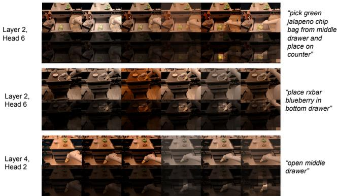
Fig. 13: In this figure we show the attention map of the RT-1 policy. Different layers and heads generally focus on different part of the image. Most commonly, they focus on the parts of the scene with the richest interaction affordances, such as graspable objects. For example, Layer 2 Head 6 focuses on the jalapeno chips and pepsi can in grasping tasks; and Layer 4 Head 2 focuses on the drawer in drawer opening tasks.
