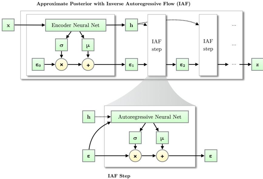
**Figure 3.1:** Like other normalizing flows, drawing samples from an approximate posterior with Inverse Autoregressive Flow (IAF) (Kingma *et al.*, 2016) starts with a distribution with tractable density, such as a Gaussian with diagonal covariance, followed by a chain of nonlinear invertible transformations of  $\mathbf{z}$ , each with a simple Jacobian determinant. The final iterate has a flexible distribution.
