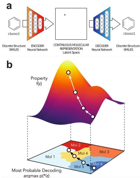
**Figure 4.2:** (a) Application of a VAE to chemical design in (Gómez-Bombarelli *et al.*, 2018). A latent continuous representation  $\mathbf{z}$  of molecules is learned on a large dataset of molecules. (b) This continuous representation enables gradient-based search of new molecules that maximizes  $f(\mathbf{z})$ , a certain desired property.
