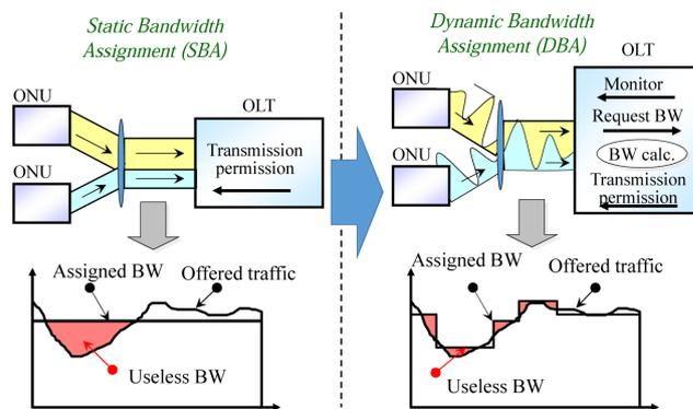
Fig. 5 Operation of DBA and non-DBA for assigned bandwidth in each ONU.
