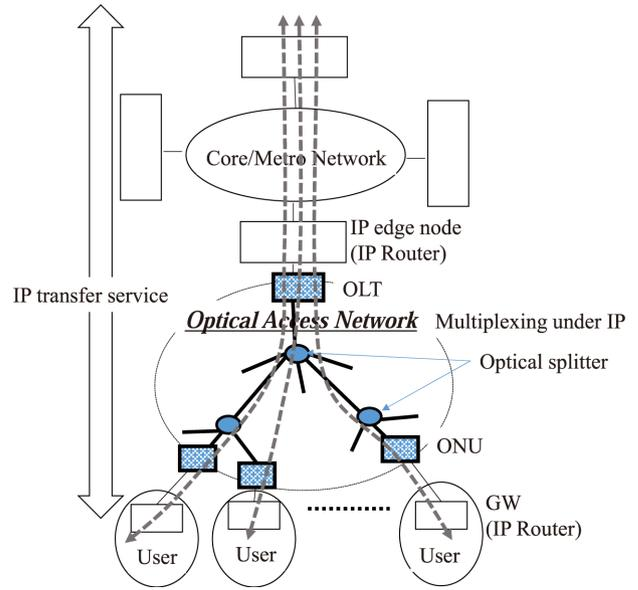
Fig. 2 Network configuration focusing on optical access network.
