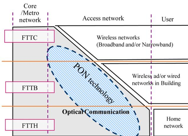
Fig. 6 PON configurations.
