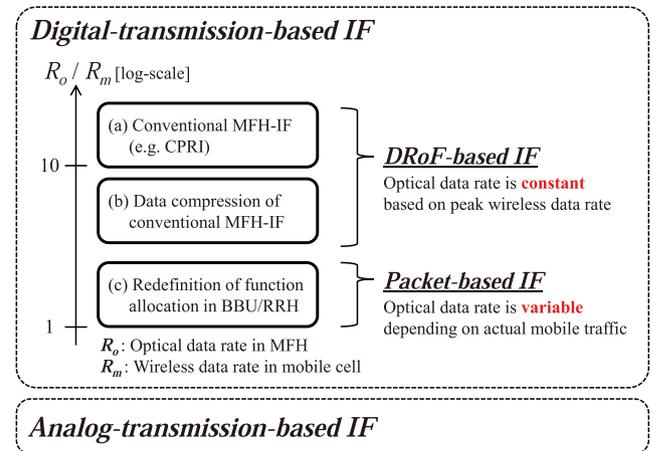
Fig. 9 Digital- and analog-transmission-based MFH interfaces.
