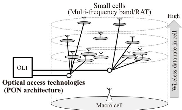
Fig. 7 Application of optical access technologies in future mobile network: PON architecture for small cells.
