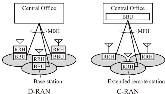
Fig. 8 D-RAN (mobile backhaul) and C-RAN (mobile fronthaul).
