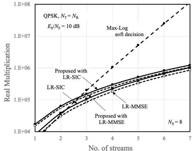
Fig. 9 Complexity of the proposed soft decoding.
