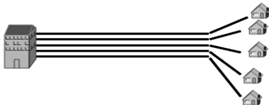
Fig. 4 Active optical network homerun architecture.
