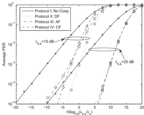
**Fig. 5** Average PER of cooperative multicell ARQ protocols when  $K = 2$ ,  $M = 2$  for symmetric multicell network. The markers '+', 'square', 'circle', and 'diamond' denote the monte carlo results of protocols I, II, III, and IV, respectively.
