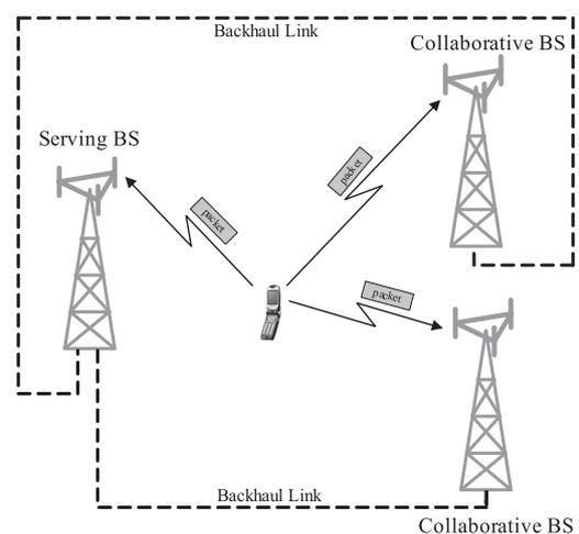
Fig. 1 Uplink CoMP for three cells.
