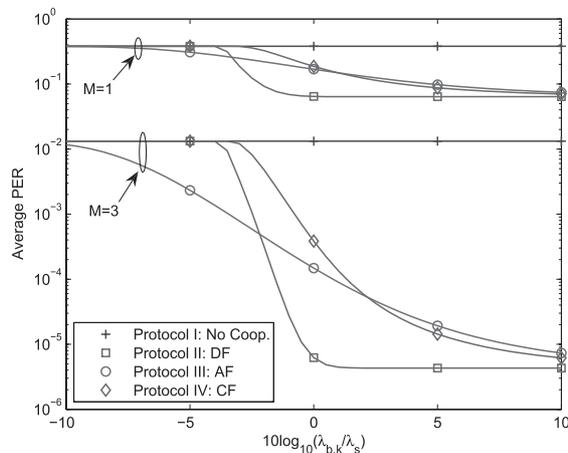
**Fig. 7** Average PER of cooperative multicell ARQ protocols when  $K = 2$  and  $\lambda_s = 10$  dB for symmetric multicell network.
