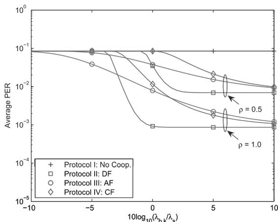
**Fig. 9** Average PER of cooperative multicell ARQ protocols when  $K = 2$ ,  $M = 2$ , and  $\lambda_s = 10$  dB, comparing the symmetric topology ( $\rho = 1.0$ ) and the asymmetric topology ( $\rho = 0.5$ ) when  $\lambda_k = \rho \lambda_s$  for all  $k$ .
