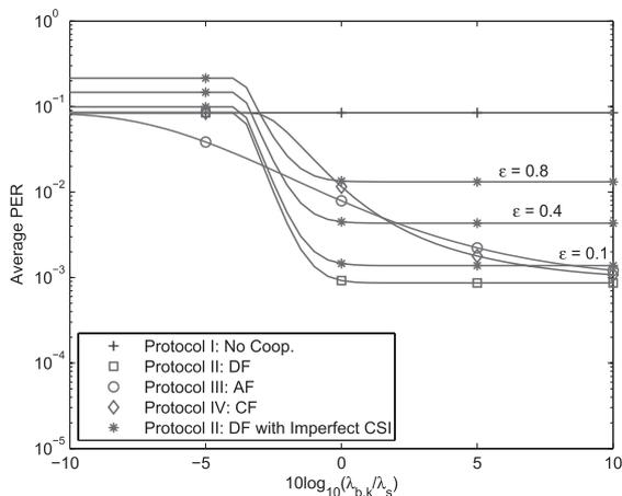
**Fig. 8** Average PER of cooperative multicell ARQ protocols when  $K = 2$ ,  $M = 2$ , and  $\lambda_s = 10$  dB for symmetric multicell network. The effect of imperfect CSI on the decoding error for ODF is reflected by setting different  $\epsilon$ .
