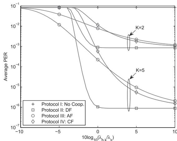
**Fig. 6** Average PER of cooperative multicell ARQ protocols when  $M = 2$  and  $\lambda_s = 10$  dB for symmetric multicell network.
