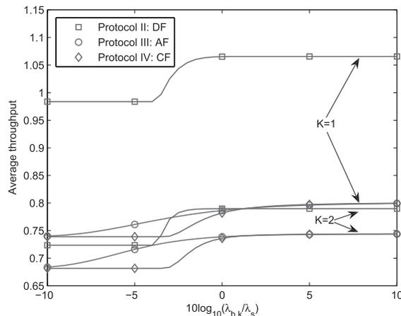
**Fig. 10** Average throughput of cooperative multicell ARQ protocols when  $M = 2$  and  $\lambda_s = 10$  dB for symmetric multicell network.
