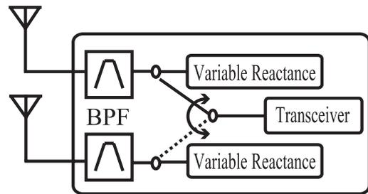
Fig. 6 SF-MIMO w/ PAE: Single Front-end MIMO with Parasitic Antenna Element.
