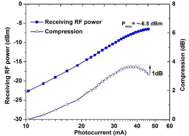
**Fig. 7** Received RF power at 60 GHz and RF compression versus average photocurrent at 5 V after 6 cm free-space transmission [28].
