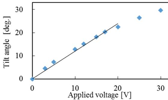
Fig. 5 Induced optical tilt angle versus the applied voltage
