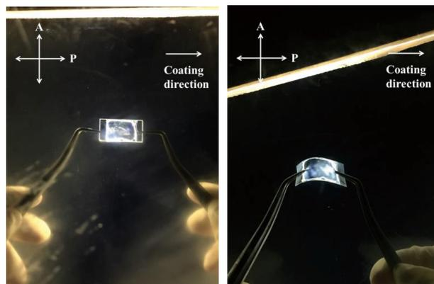
**Fig. 2** Aspects of the ULH LCD where PC films were used as the substrate
