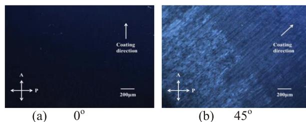
**Fig. 3** Microphotographs of the ULH texture after bending and removal from the electrical field. (a) The coating direction is parallel to the analyzer. (b) The coating direction is 45° with respect to the analyzer.
