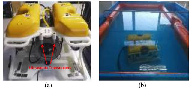
Fig. 4 The experiment system of measuring thickness of oil slick.
