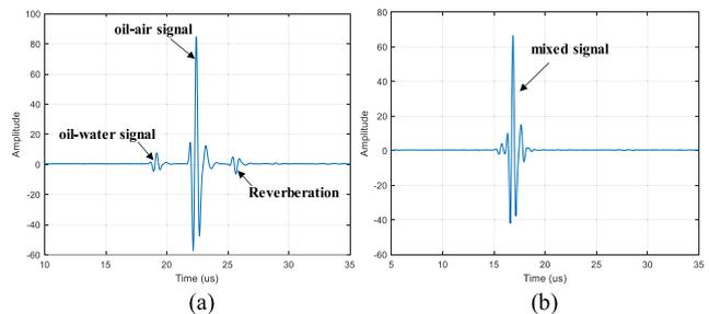
Fig. 5 The measurement echoes of the oil slick.
