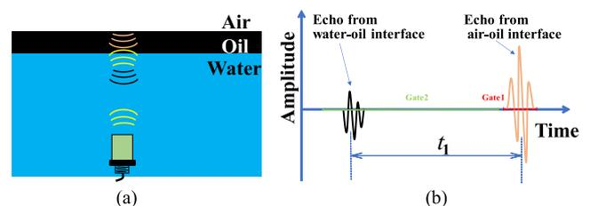
Fig. 1 The measurement schematic of the oil slick thickness.
