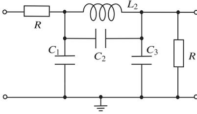
**Fig. 1** 3rd order LC ladder filter with elliptic function.
