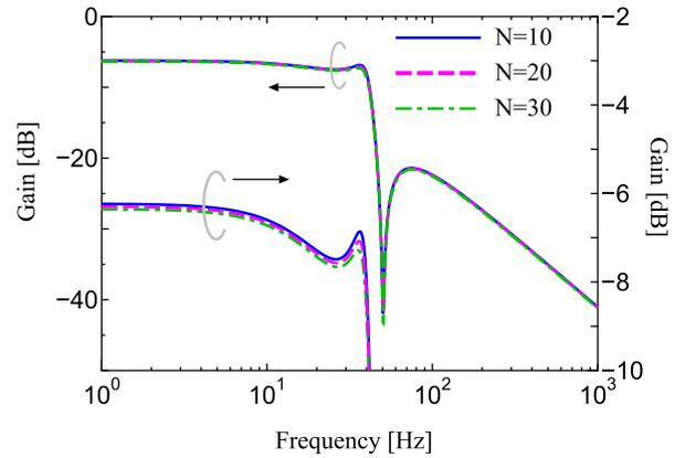
Fig. 13 Gain of low-pass notch filters with varying scaling factor.
