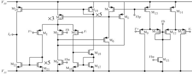
**Fig. 2** Circuit configuration of OTA.
