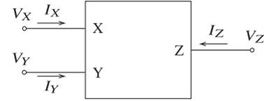
**Fig. 3** Block diagram of CCII.
