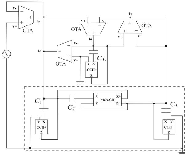
Fig. 6 Active 3rd order low-pass notch filter employing CCII based capacitance multipliers.
