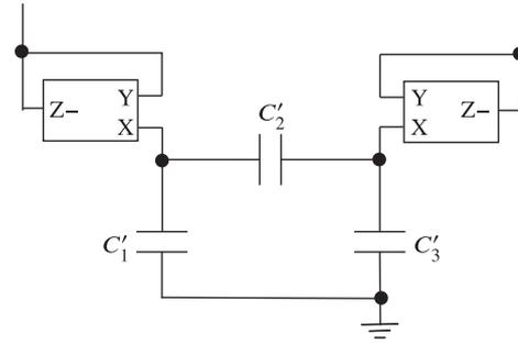
Fig. 7 Proposed technique to reduce capacitance multipliers.
