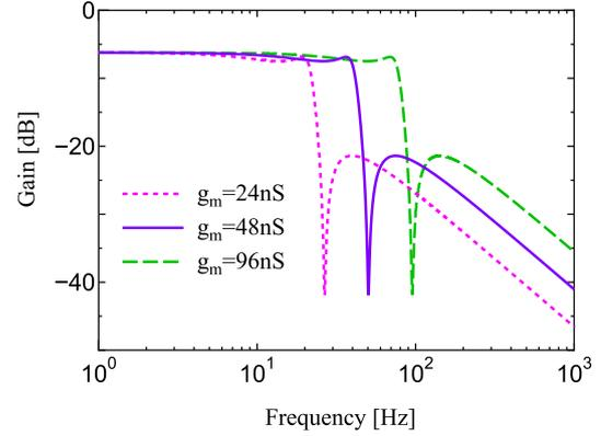
Fig. 12 Tuning cutoff frequency of low-pass notch filter.
