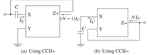
**Fig. 4** Grounded capacitance multipliers constructed of a CCII.
