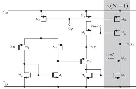
Fig. 9 Circuit configuration of CCII+.
