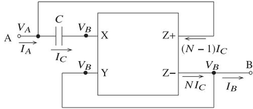
Fig. 5 Floating capacitance multiplier constructed of an MOCCII.
