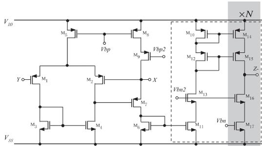
Fig. 10 Circuit configuration of CCII-.
