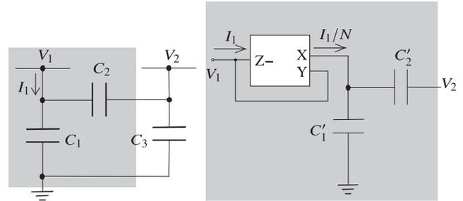
Fig. 8 Corresponding part in capacitor network
