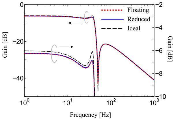
Fig. 11 Gain of frequency characteristics of low-pass notch filters.
