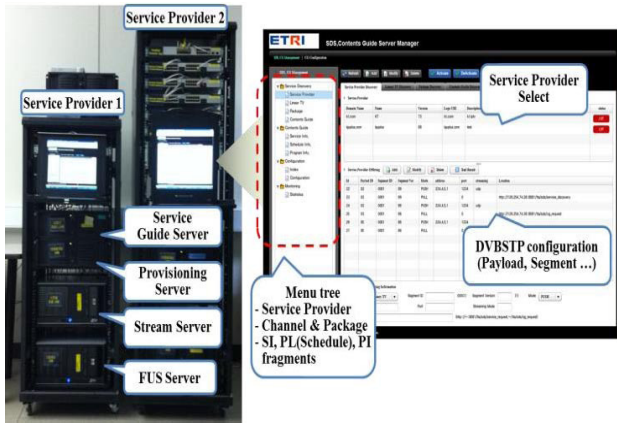
Fig.9 IPTV server RI and web based management UI to configure the encapsulation and delivery environments.
