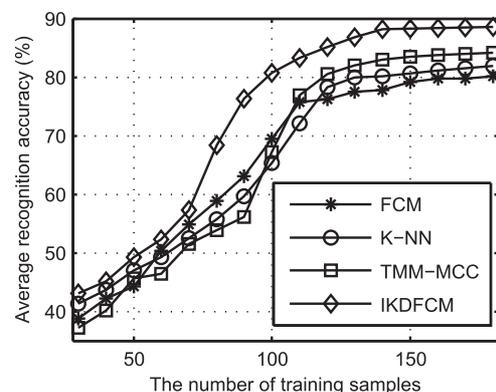
Fig. 3 The recognition rate versus the number of training samples when SNR = 35dB.
