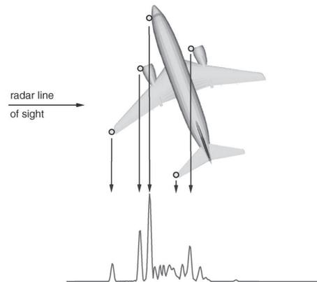
**Fig. 1** HRRP of an aircraft, it shows the discriminative information on the geometry of aircraft. This figure is cited from [5].
