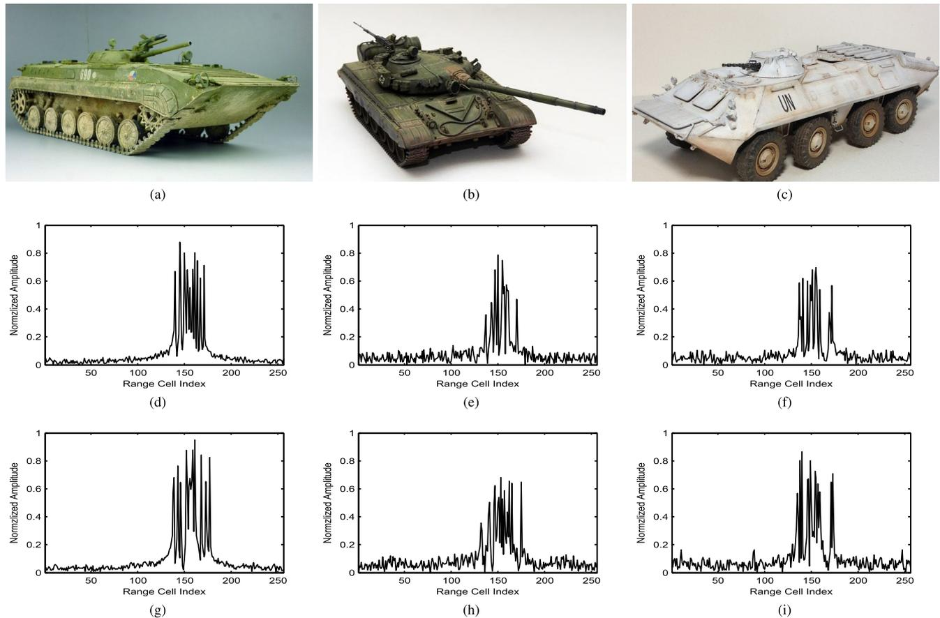
**Fig. 2** The optical images [33] and the HRRP of the three targets. (a) the optical image of BMP2; (b) the optical image of BTR70; (c) the optical image of T72; (d)–(f) the HRRP of the corresponding three targets above when the azimuth is 30°; (g)–(i) the HRRP of the corresponding three targets above when the azimuth is 60°.
