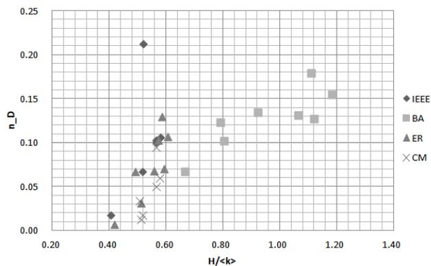
**Fig. 6** Plot of  $n_D$  as a function of  $H/\langle k \rangle$  for power grids and their corresponding ER, BA and CM networks.
