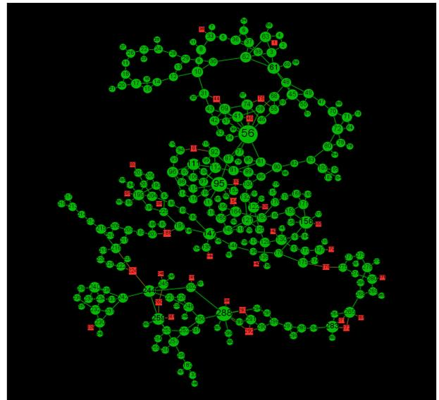
Fig. 4 The topology of the Middle China power grid (MC302), where squared nodes denote the controllers.
