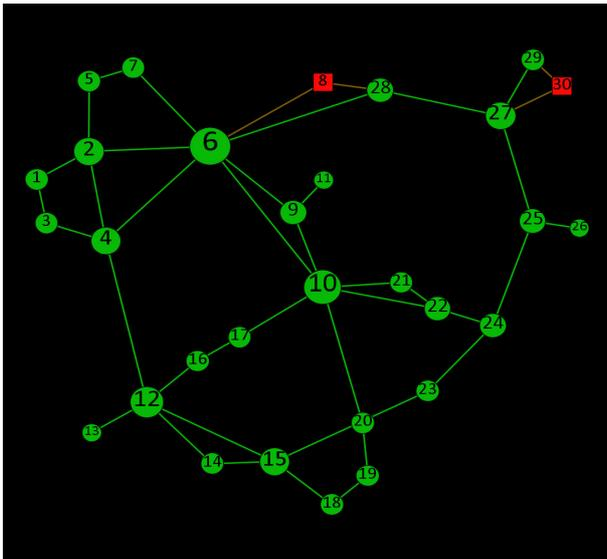
Fig. 2 The topology of the IEEE30 power grid, where squared nodes denote the controllers.
