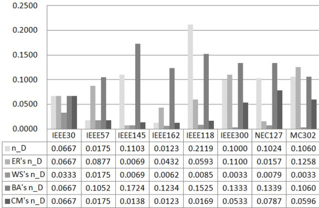
Fig. 1 Comparisons of the controllability values between all power grids and corresponding ER, WS, BA and CM network models.
