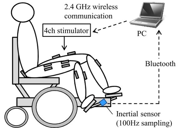
Fig. 2 Experimental setup of FES cycling control tests with the cycling wheelchair “Profhand”.
