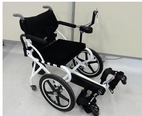
**Fig. 1** Cycling wheelchair “Profhand” (TESS Co., Ltd.) used in the experiments.
