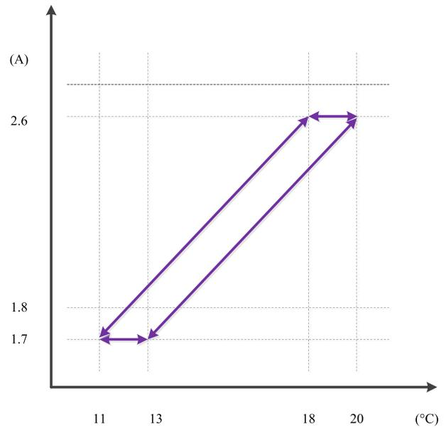
**Fig. 6** Hysteresis curve for the charging current control in the [11°C–20°C] range.
