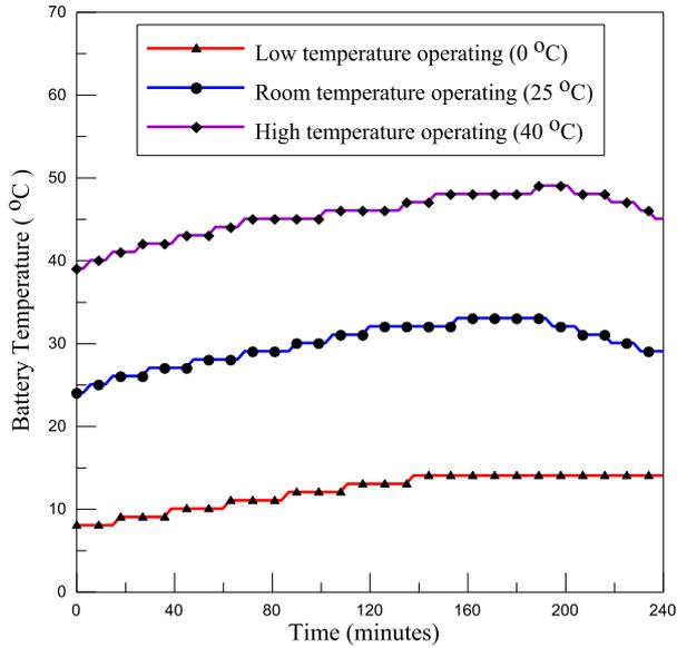
**Fig. 10** Battery temperature changes during different environmental temperatures.
