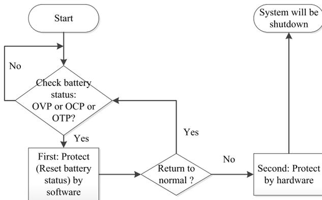
Fig. 15 Flowchart of battery protect by software and hardware.
