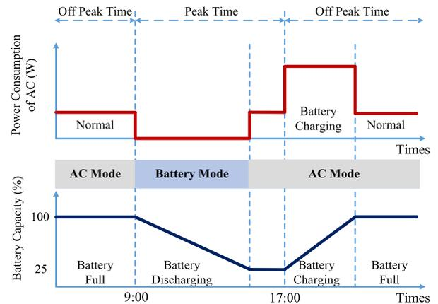
Fig. 4 Power consumption of the peak-shift control method.
