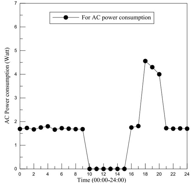
Fig. 8 AC power consumption measurements of the peak-shift control method.
