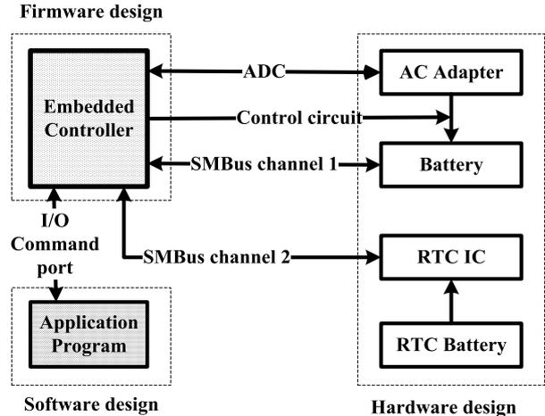
Fig. 2 System architecture of the EC and application program.
