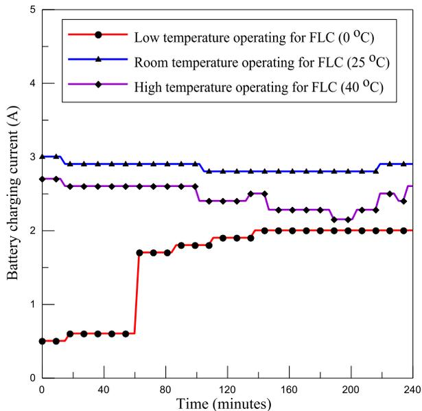
**Fig. 11** The battery charging current for FLC during different environmental temperatures.
