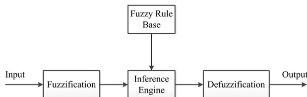
Fig. 1 Structure of the fuzzy logic system.
