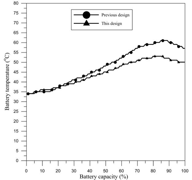
**Fig. 12** The battery temperature variation measurement with respect to battery charging capacity of the previous design and of this design.
