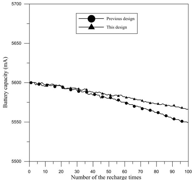
**Fig. 13** Full battery capacity with respect to the number of the recharging times for the previous design and this design.
