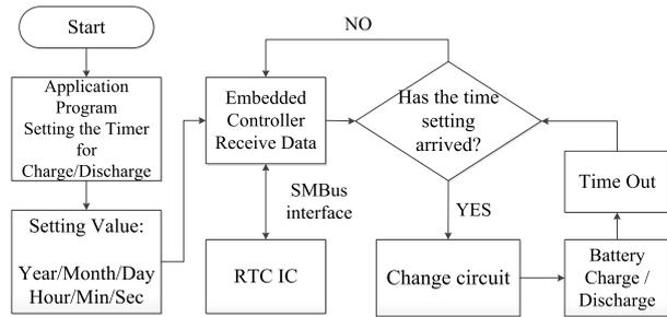
Fig. 3 Flowchart of the peak-shift control method.
