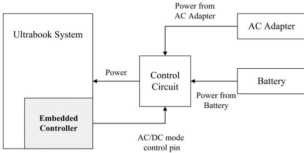
Fig. 7 AC/DC power supply controlled by the EC.
