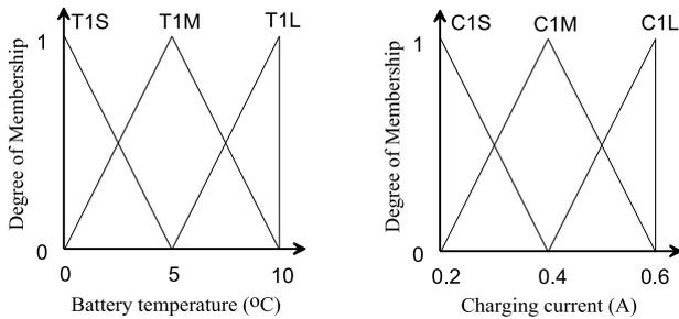
**Fig. 5** Membership function of the battery temperature [0°C–10°C] and the charging current [0.2A–0.6A].
