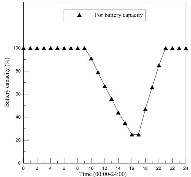
Fig. 9 Battery capacity measurements of the peak-shift control method.
