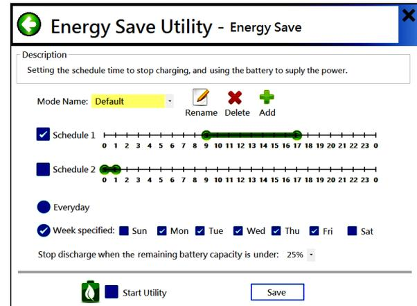
Fig. 17 The user peak-shift function setting.
