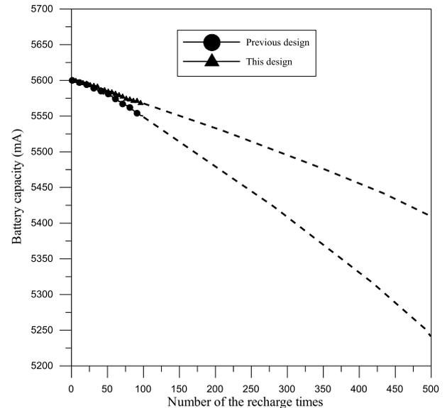
**Fig. 14** Battery capacity with respect to the number of the recharging times from the measurement result to the prediction result.
