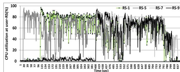
**Fig. 2** CPU trace on 9RSs of bulk loading 10 million records.
