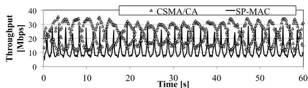
**Fig. 7** Time evolution of the total throughput for both AP's when the terminals use CUBIC-TCP (CSMA/CA, original SP-MAC).
