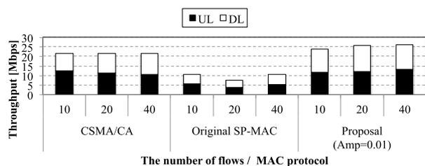
Fig. 9 The throughput of UL and DL at AP1 (CUBIC-TCP).
