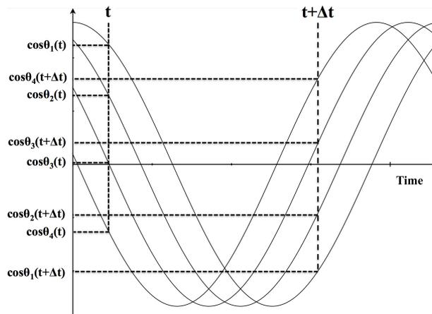
Fig. 1 Example: cosine curves of synchronized oscillators with phase shifting.
