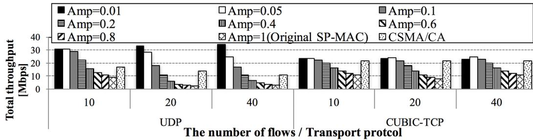
Fig. 3 Total throughput for each  $Amp$  value and number of flows.
