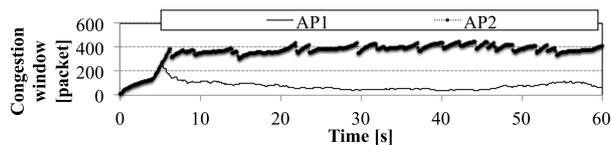
**Fig. 4** The total congestion window size of all wireless terminals of connected each APs (CSMA/CA).
