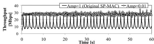
**Fig. 8** Time evolution of total throughput for all APs for each  $Amp$  value when the terminals use CUBIC-TCP ( $Amp = 1$ : original SP-MAC,  $Amp = 0.01$ ).
