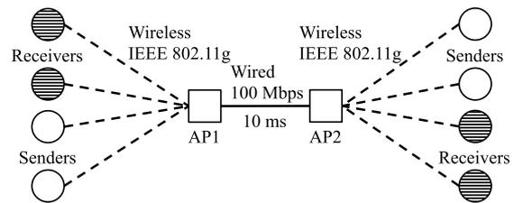
Fig. 2 Network model for the evaluation.
