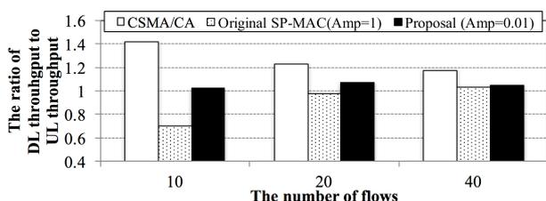
Fig. 10 The ratio of DL throughput to UL one at AP1 (CUBIC-TCP).
