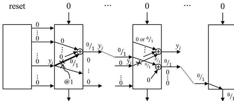
Fig. 14 LFSR testing for feedback line  $(y_i - y_j)$  s-a-1 fault.
