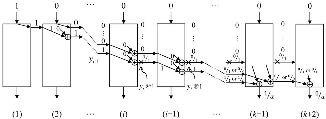
Fig. 8 LF²SR testing for  $y_i$  s-a-1 fault.
