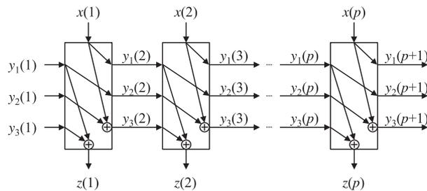
**Fig. 3** Time expansion model of  $R_1$ .
