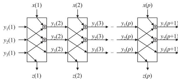
**Fig. 4** Time expansion model of  $R_2$ .
