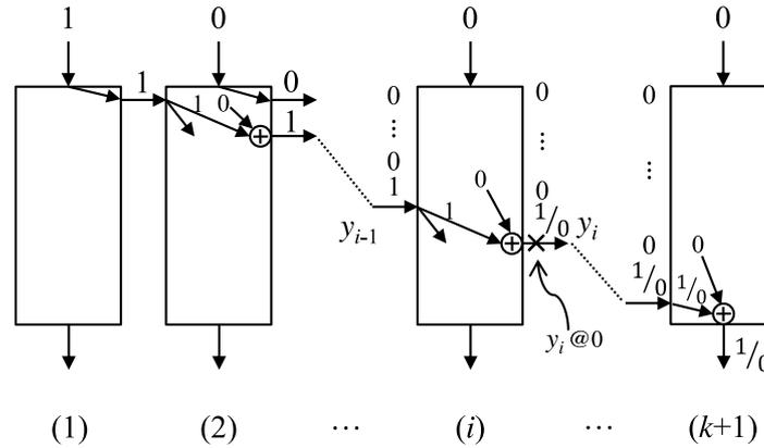
Fig. 7 LF²SR testing for  $y_i$  s-a-0 fault.
