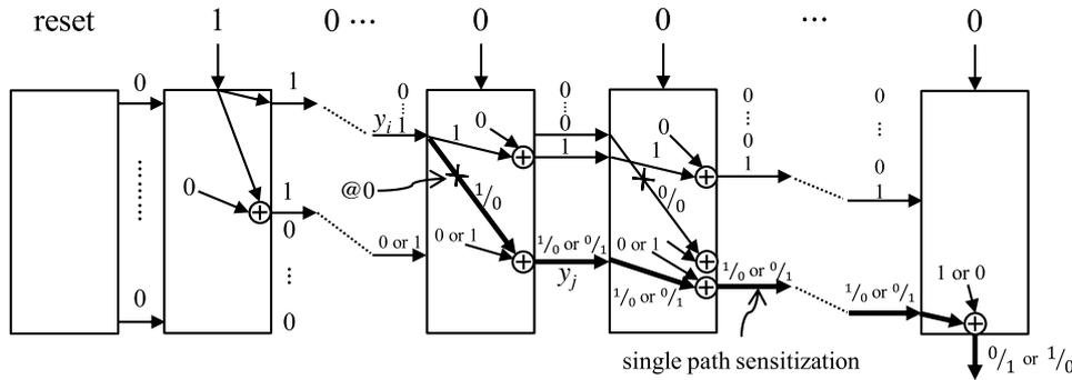
Fig. 9 L<sup>2</sup>SR testing for feed-forward line  $(y_i - y_j)$  s-a-0 fault.
