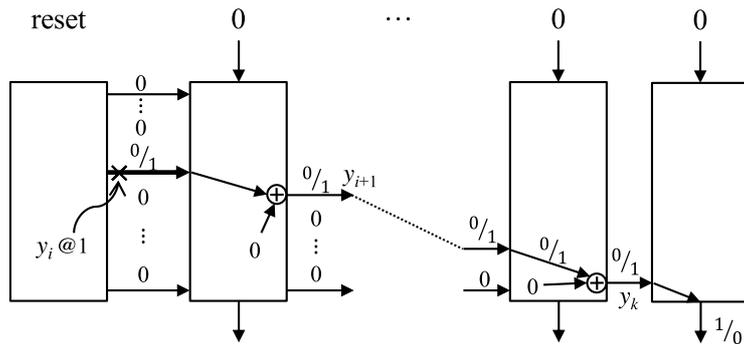
Fig. 13 LFSR testing for  $y_i$  s-a-1 fault.
