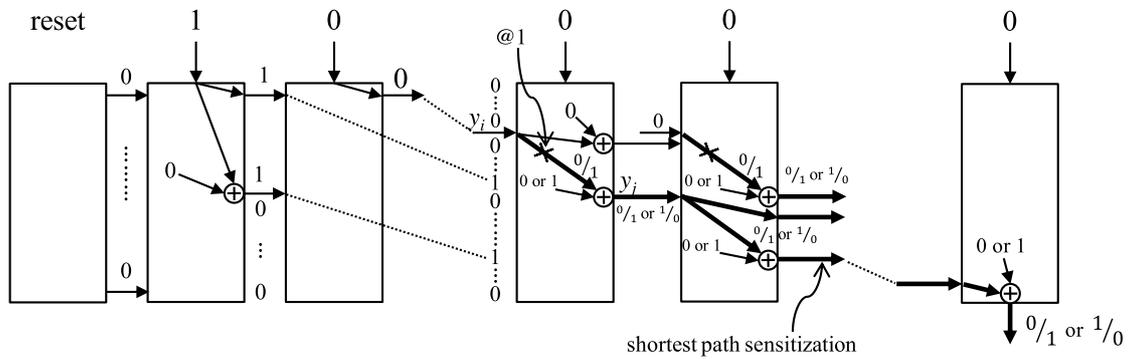
Fig. 10 L<sup>2</sup>SR testing for feed-forward line  $(y_i - y_j)$  s-a-1 fault.
