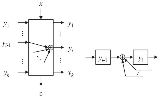
Fig. 6 Structural characteristics of LFSRs.
