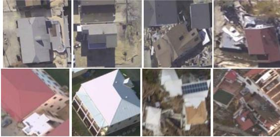
**Fig. 3** Examples of datasets Sandy and Irma. The first row denotes samples of Sandy dataset, the second row denotes images of Irma dataset. The first and second columns indicate samples of undamaged buildings, the third and fourth are the samples of damaged buildings.
