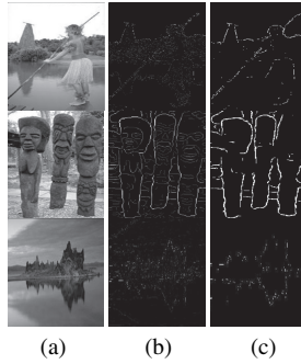
Fig. 3 Results of salient point detection. Column (a) are the original images, column (b) are edge detection result of SSE, and column (c) are the final result of tensor voting—salient point detection images.
