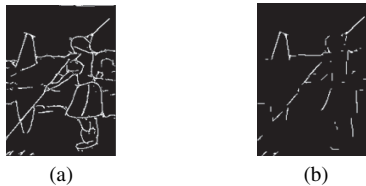
Fig. 6 Boundary detection image and salient edge image. (a) is a boundary detection image, (b) is a salient edge detection image.
