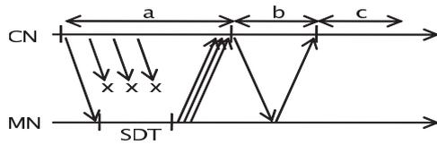
Fig. 5 Three sections where timeout interval can fall.
