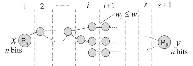
Fig. 1 Network  $G$  that is partitioned into  $(s+1)$ -layers.
