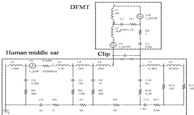
Fig. 2 The equivalent electrical model regarding the lumped mechanical models of the human middle ear, coupled with the DFMT.
