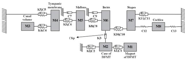
Fig. 1 Lumped mechanical models of the human middle ear coupled with the DFMT.
