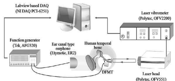
Fig. 5 Block-diagram of experimental setup.
