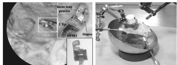
Fig. 4 Photograph of vibration measurement setup and DFMT attached to the incus long process.
