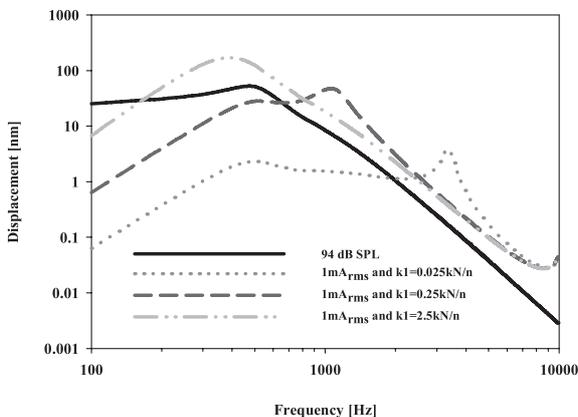
Fig. 3 The simulated stapes displacement in both cases of the DFMT unloaded and the loaded states under different conditions.
