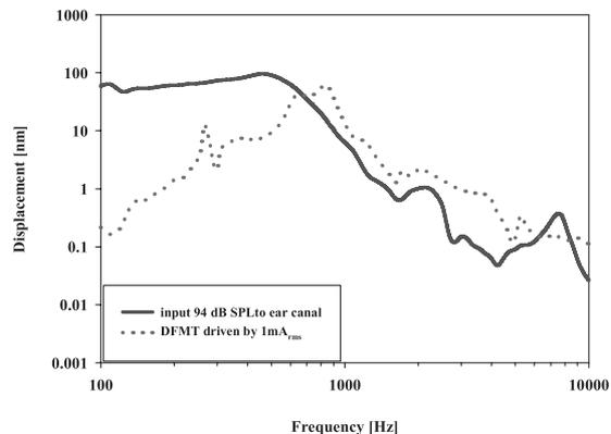
**Fig. 6** The measured stapes displacements in regards to the in-vitro experiment by using the human temporal bones and the DFMT.
