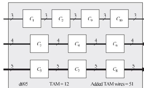
**Fig. 11** Dedicated test bus design with 12-bit TAM for *d695*.
