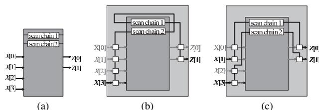
**Fig. 12** Wrapper for transparency-based SoC test. (a) Original core. (b) Wrapper for *INTEST* with 1-bit access. (c) Wrapper for *INTEST* with 2-bit access.
