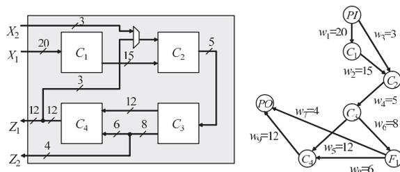
**Fig. 3** Acyclic SoC and its system graph  $G$  for the example SoC  $S_1$ .
