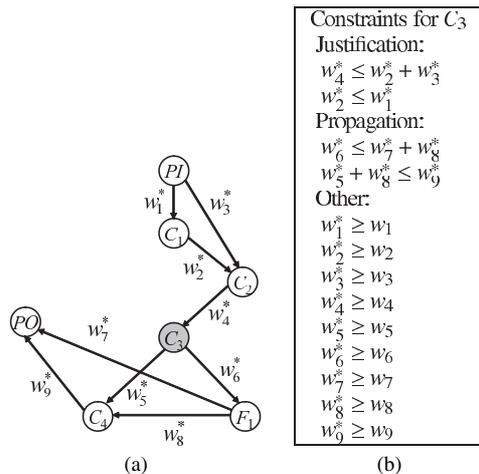
**Fig. 4** (a) Test graph  $G_3$ . (b) Constraints on the edge weights for  $C_3$  in [23].
