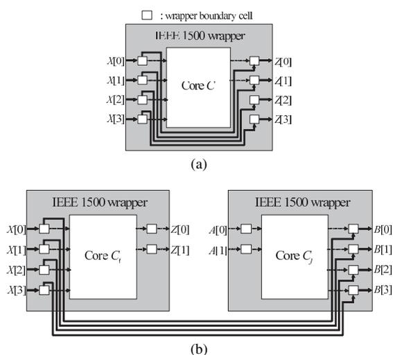
**Fig. 6** (a) Single-core bypass path by IEEE 1500 wrapper. (b) Multi-core bypass path by IEEE 1500 wrapper.
