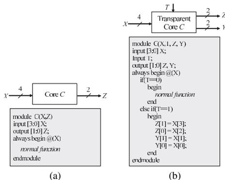
**Fig. 1** Embedding a multiplexer in the behavioral description. (a) Original core. (b) Core with embedded multiplexers.
