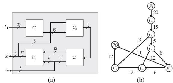
**Fig. 2** An example SoC  $S_1$  and its system graph.
