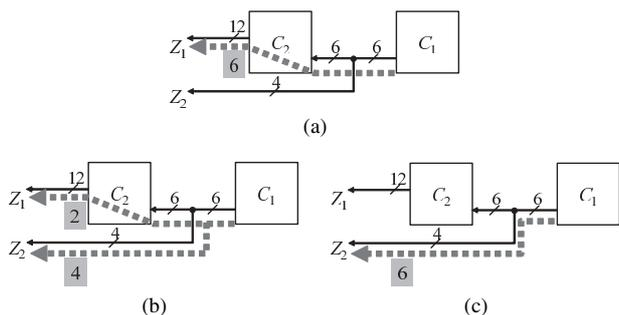
**Fig. 5** Propagation paths in various costs for transparency. (a) Cost for making  $C_2$  1-bit transparent is 0. (b) Cost for making  $C_2$  1-bit transparent is 1. (c) Cost for making  $C_2$  1-bit transparent is 2 and cost for 1-bit additional interconnect on  $Z_2$  is 1.
