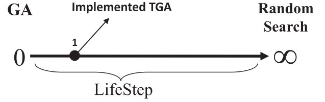
Fig. 5 The TGA algorithm acts like GA or random search algorithm by adjusting LifeStep parameter.
