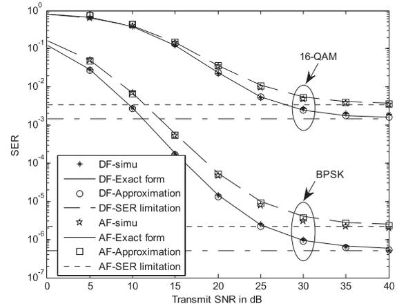
**Fig. 4** Theoretical and simulation results of the SER for both DF and AF cooperative systems with one relay. Different modulations are considered and  $\alpha = 0.01$ .
