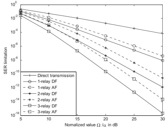
**Fig. 5** Limitation of the SER when  $P/N_0 \rightarrow \infty$  for the DF and AF cooperative systems with different number of relays versus the normalized value  $\Omega/\alpha$ .
