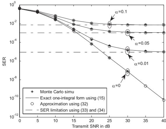
**Fig. 2** Theoretical and simulation results for the SER of the DF cooperative system with one relay using 4-QAM signals. The variance of channel estimation errors is fixed as  $\alpha \in \{0.1, 0.05, 0.01, 0\}$ .
