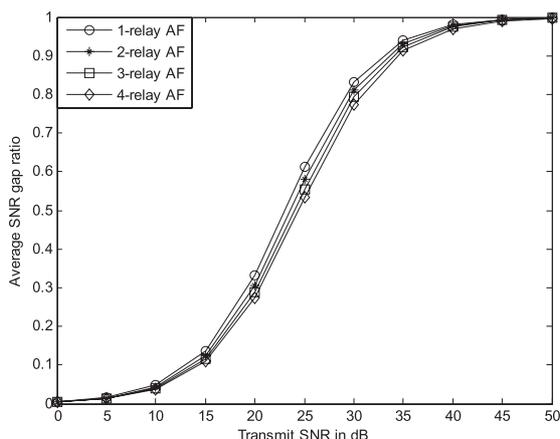
**Fig. 7** Average SNR gap ratio of the AF cooperative system with different number of relays versus the transmit SNR. The variance of channel estimation errors is fixed as  $\alpha = 0.01$ .
