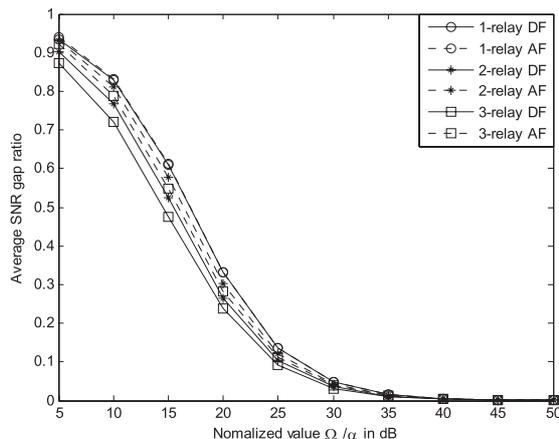
**Fig. 8** Comparison of the average SNR gap ratio between the DF and AF cooperative systems with different number of relays versus the normalized value  $\Omega/\alpha$ . The transmit SNR is fixed as  $P/N_0 = 20$  dB.
