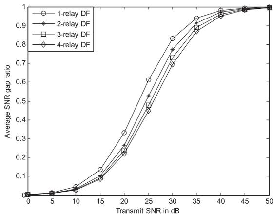
**Fig. 6** Average SNR gap ratio of the DF cooperative system with different number of relays versus the transmit SNR. The variance of channel estimation errors is fixed as  $\alpha = 0.01$ .
