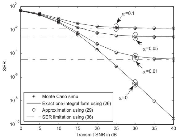
**Fig. 3** Theoretical and simulation results for the SER of the AF cooperative system with one relay using 4-QAM signals. The variance of channel estimation errors is fixed as  $\alpha \in \{0.1, 0.05, 0.01, 0\}$ .
