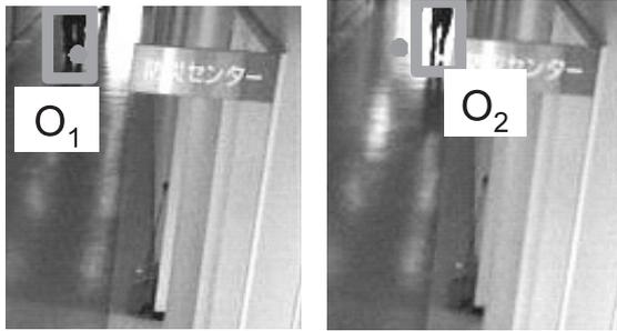
**Fig. 16** Results of object detection and tracking. These images are the partial images of  $C_1$  (right-upper partial images). Rectangles indicate detected objects. The centroids of objects  $O_1$  and  $O_2$  were regarded as the positions of IN/OUT data. Such varying positions are merged into the end point of a route (i.e. the mean position,  $\mu_r^B$  or  $\mu_r^E$ , of route  $r$ ). The end point is indicated by an orange circle in the figure.
