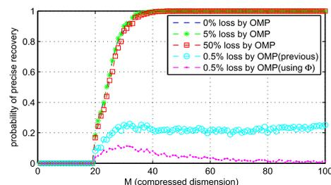
**Fig. 1** Data recovery by OMP with  $\hat{\Phi}$  for data loss rates  $(1 - P)$  of 0%, 5%, 50%, comparing with OMP using  $\Phi$  instead of  $\hat{\Phi}$  or OMP with previous readings ( $N = 100$ ,  $K = 9$ ).
