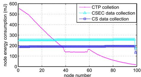
**Fig. 3** Energy consumption of every sensor node in the network under 20% packet loss. CS data collection is more balanced than CTP, and CSEC consumes more energy than our CS.
