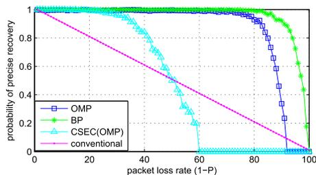
**Fig. 2** Compare our proposed method with two different data recovery approaches. (1) CS with OMP and BP respectively ( $M = 40$ ,  $K = 9$ ), (2) CSEC [3] with OMP ( $M = 48$ ,  $K = 9$ ), (3) conventional aggregation.
