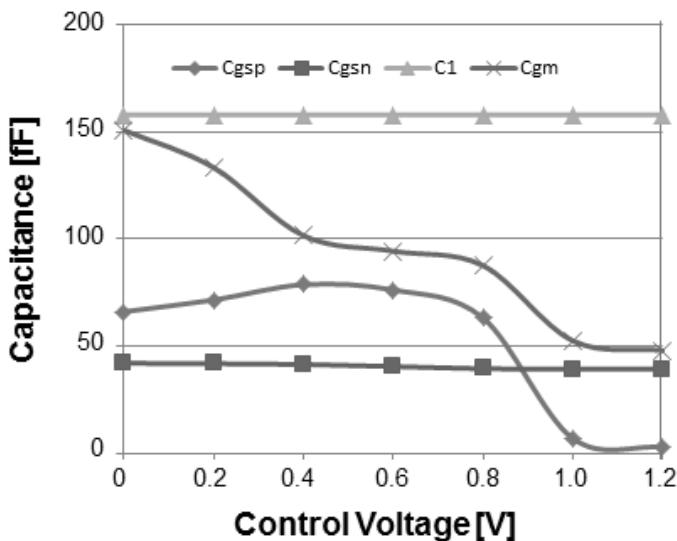
**Fig. 3.** Simulated capacitance characteristics for the VCO circuit
