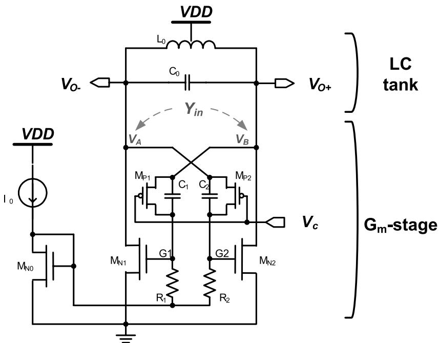
Fig. 1. LC-VCO circuit without a varactor device
