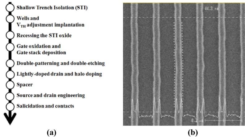
**Fig. 1.** (a) Sequence of the front-end-of-line CMOS fabrication process, (b) Plane view of the SEM image from a test structure that investigates the LER profile.
