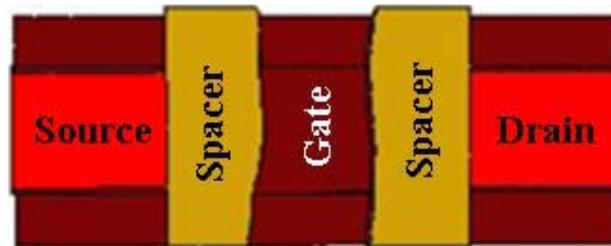
**Fig. 2.** Top view of the n-type QPT bulk MOSFET with a 2P2E-LER experimental profile. The gate electrode is not shown to clearly depict the LER profiles on both sides next to the spacer. In this study,  $W_{eff}/L_{eff} = 60/36$  nm.
