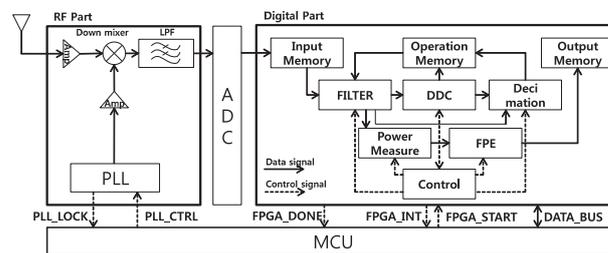
Fig. 1. A circuit diagram of the proposed digital spectrum sensor.
