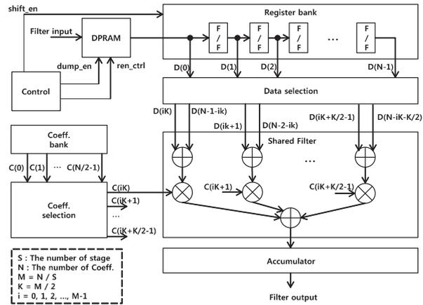
Fig. 2. A block diagram of the proposed FIR filter.
