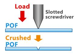
Fig. 1. Processing procedure of the crushed polymer optical fiber (POF).
