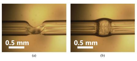
Fig. 3. Micrographs of the crushed polymer optical fiber: (a) side view and (b) top view.
