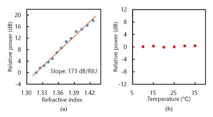
Fig. 4. (a) Measured relative transmitted power dependence on the refractive index (RI). (b) Relative transmitted power dependence on temperature when the refractive index was 1.366.
