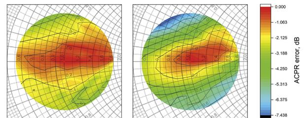
Fig. 4. Comparison of ACPR error between POLDPD and traditional off-line DPD with  $\lambda = 0.05 \text{ V}^{-1}$  (left) and  $\lambda = 0.5 \text{ V}^{-1}$  (right).
