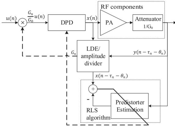
Fig. 1. Proposed on-line DPD structure.
