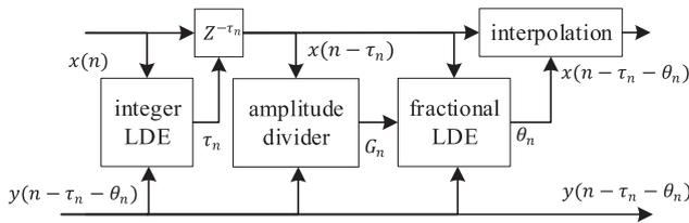
Fig. 2. LDE and amplitude divider structure with real-time processing.
