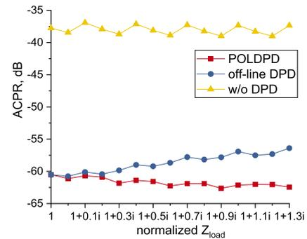
Fig. 3. ACPR performance comparison along with the imaginary part of load impedance increasing.
