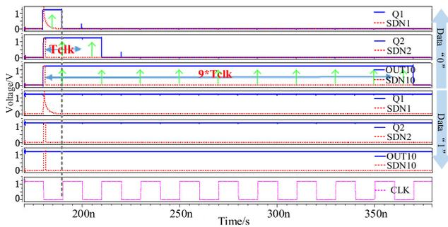
Fig. 9 Simulation results of injecting a pulse into the SDN node.
