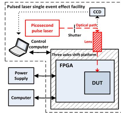
Fig. 2 Principle block diagram of the experimental setup.
