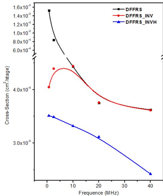
Fig. 5 SEU cross-section vs. frequency of the DFFRS, DFFRS\_INV, and DFFRS\_INVH chains.
