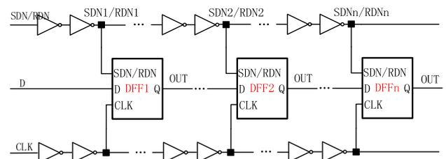
Fig. 8 Circuit structure diagram of the DFF chain.
