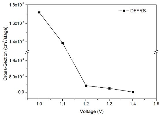
Fig. 4 SEU cross-section of the DFFRS chain versus the supply voltage.
