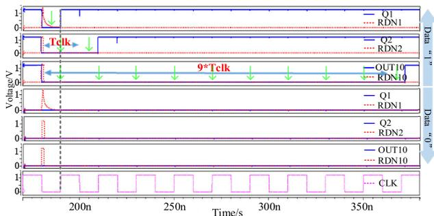
Fig. 10 Simulation results of injecting a pulse into the RDN node.
