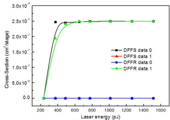
Fig. 7 SEU cross-section vs. laser energy of the DFFS and DFFR chains in data “0” and data “1” test.
