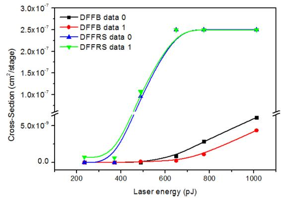
Fig. 6 SEU cross-section vs. laser energy of the DFFB and DFFRS chains in data “0” and data “1” tests.
