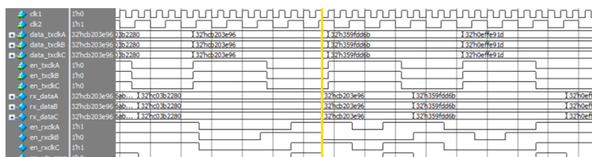
Fig. 9 Oscillogram of DMUX with metastable injection.
